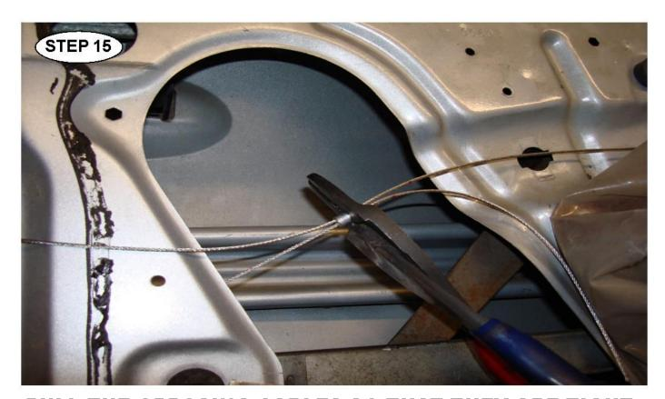
PULL THE OPPOSING CABLES SO THAT THEY ARE TIGHT (BUT NOT ENOUGH TO PULL THE LEVER OF THE LATCH). BACK OUT ONE OF THE CABLES FROM THE ABOUT 3/8", JUST TO GIVE A LITTLE SLACK. CRIMP THE FERRULE. CRIMP A FEW TIMES ACROSS THE ENTIRE LENGTH OF THE FERRULE TO ENSURE THAT THE CABLE DOES NOT COME LOOSE. CLOSE THE DOOR AND TEST THE HANDLE MAKING SURE IT OPENS THE LATCH. CUT OFF EXCESS CABLE. REPEAT THESE STEPS FOR THE PASSENGER DOOR AND THEN REINSTALL DOOR PANELS.
