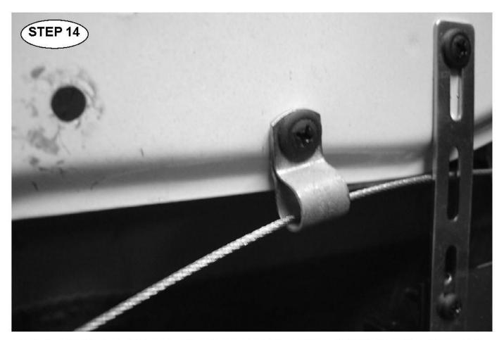
MAKE SURE THAT THE CABLE IS NOT GOING TO RUB ON THE ACTUATOR. IF IT IS, USE THE SUPPLIED GUIDES TO RELOCATE THE CABLE.
