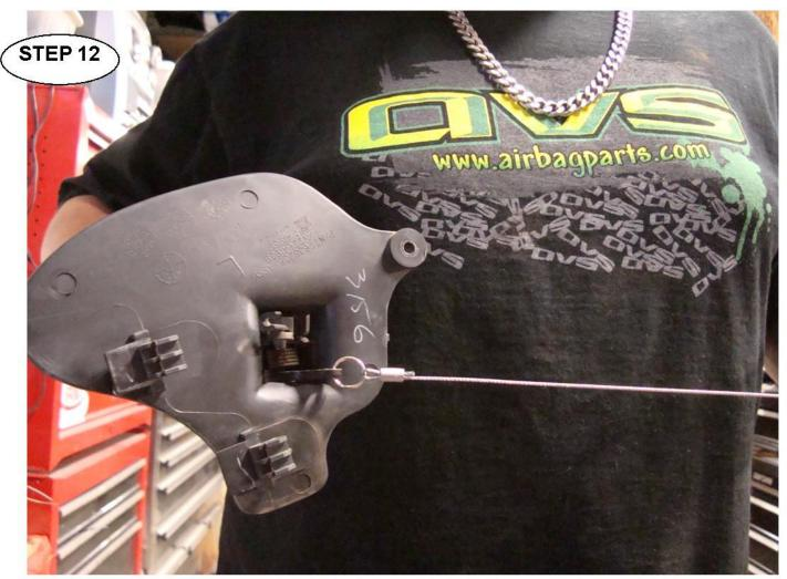
CONNECT THE ONE OF THE RINGS THAT HAS ONLY A SINGLE CABLE TO THE EYELET ON THE BACK OF THE INTERIOR DOOR HANDLE. NOW INSTALL THE HANDLE BACK ONTO THE DOOR LEAVING THE CABLE OUT WHERE YOU HAVE ACCESS TO IT.
