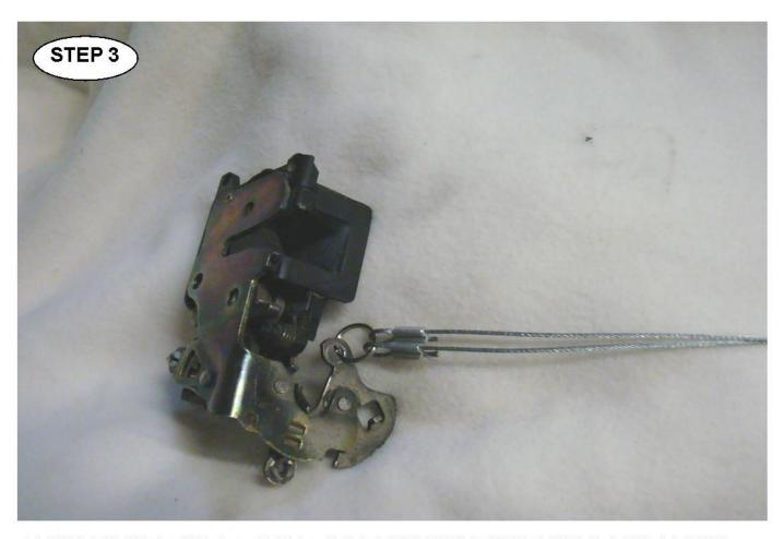
NOW TAKE THE CABLE ASSEMBLY THAT HAS THE TWO CABLES WITH THE "KEY CHAIN" STYLE CONNECTING RING AND LOOP THE CONNECTING RING TO THE PART OF THE LATCH WHERE THE INTERIOR DOOR HANDLE WAS ONCE CONNECTED. NOTE: IF YOUR LEVER HAS 2 OR MORE HOLES, ALWAYS USE THE HOLE THAT IS LOCATED AT THE HIGHEST POINT AS IN THE PICTURE ABOVE.
