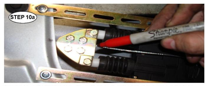
WITH A MARKING PEN, MAKE A MARK ON THE CABLE DIRECTLY BEHIND THE CLAMPING PLATE. AGAIN, MAKE SURE THAT THE DOOR OPENS ON EVERY TRY OF THE REMOTE BEFORE MOVING TO THE NEXT STEP.
