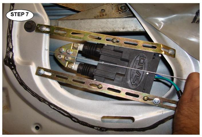
IF THE OPENING OF THE DOOR CAVITY IS TOO BIG, SECURE THE 9" METAL STRAPS TO THE ACTUATOR PACK WITH THE SUPPLIED 1" BLACK SCREWS, AND THEN SCREW THE 1/2" SELF DRILLING SCREWS THROUGH THE STRAPS AND INTO THE DOOR USING A POWER SCREWDRIVER.
