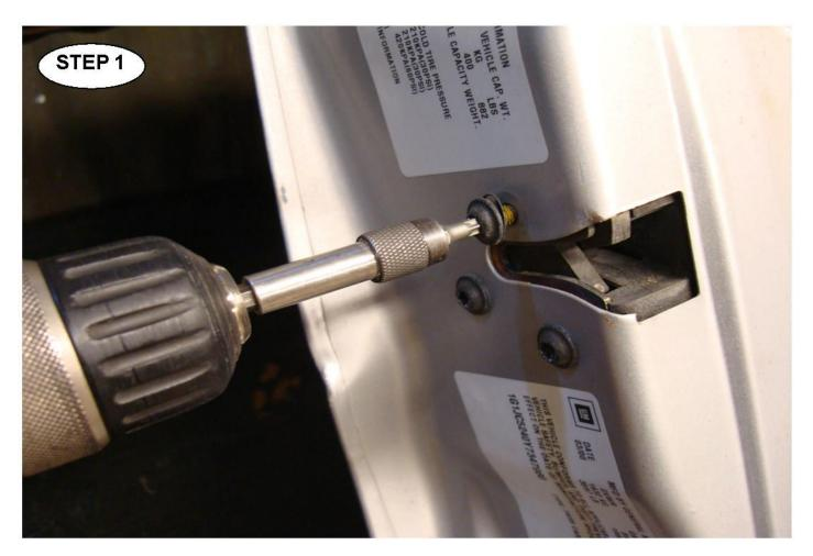
LEAVE THE WINDOW DOWN ON THE DOOR THAT IS NOT BEING WORKED ON. THIS WILL PREVENT YOU FROM LOCKING YOURSELF OUT OF THE VEHICLE. ON THE DOOR THAT YOU ARE WORKING ON, LEAVE THE WINDOW ROLLED UP. REMOVE THE INTERIOR DOOR PANELS FROM THE VEHICLE. REMOVE THE SCREWS THAT HOLD THE LATCH TO THE DOOR.
