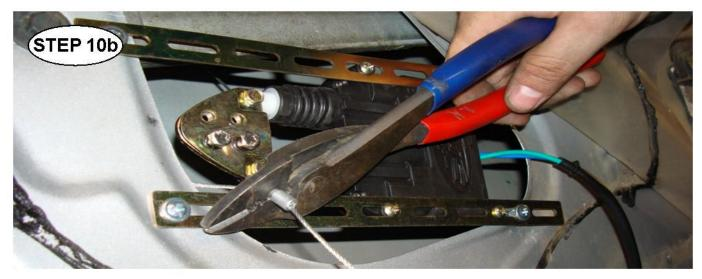
LOOSEN THE CLAMPING PLATE BOLTS AND REMOVE THE CABLE. TAKE ONE OF THE ALUMINUM CRIMP FERRULES AND SLIDE IT OVER THE CABLE AND STOP WHEN YOU REACH THE MARK THAT YOU MADE. NOW CRIMP IT DOWN WITH A CRIMPING OR SWAGING TOOL.
