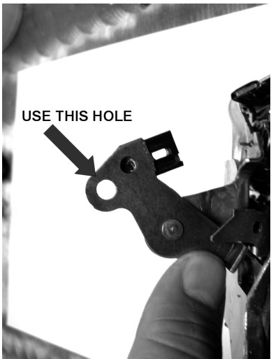
7. INSTALL THE BOLT THROUGH THE LOOP OF THE ACTUATOR CABLE AND THROUGH THE CLOSEST HOLE ON THE LEVER ABOVE IT. FINGER TIGHTEN THE LOCK NUT. TIGHTEN THE BOLT AND NUT BY HOLDING THE LOCK NUT WITH PLIERS AND USING A WRENCH OR 5/32" SOCKET TO TURN THE BOLT.
